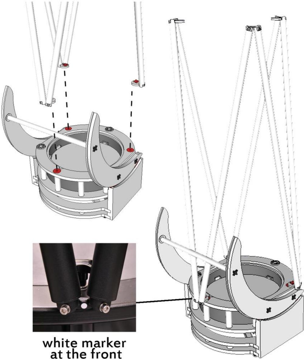
Step 5. We put the top cell on the truss, the screws should partially fall into the hole for easy installation. The screw that is nearest to the focuser should be at the back of the telescope. Screw in and tighten the screws at the top cell, and then tighten the screws at the bottom of the truss.
